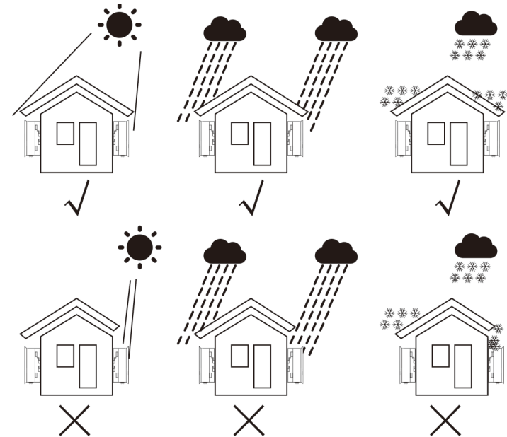
▲ Figure 5.1 Recommended installation position
